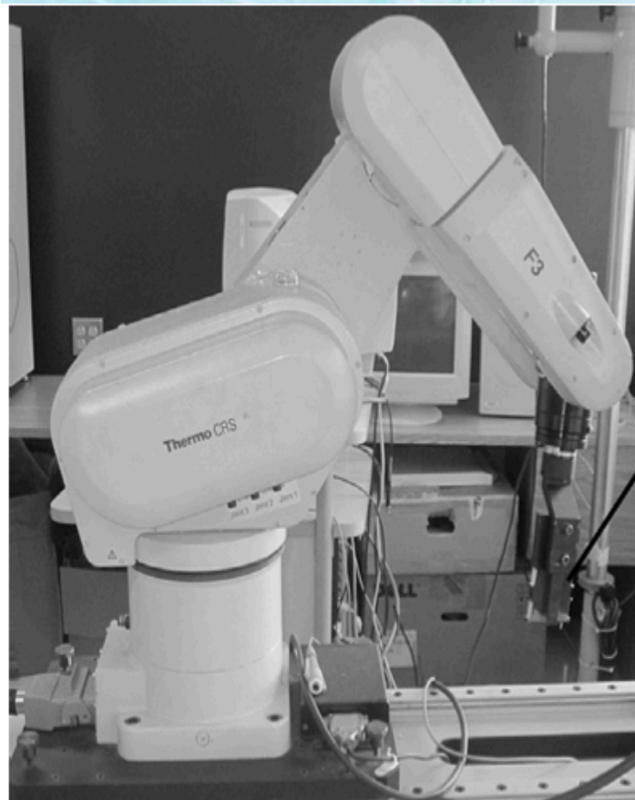
Fig. 1. F3 CRS robotic arm used in the 3-D ultrasound (US) imaging robotic system.
