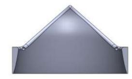
Two sections of housing structure a) housing inner profile at the section parallel to leaflets axis of rotation b) housing inner profile at the section perpendicular to leaflets axis of rotation
