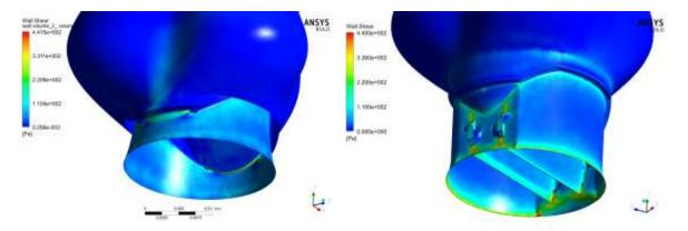
Wall shear stress in valve region a) in newly designed valve with lower values in hinge area b) in a conventional bileaflet valve with higher values in hinge area
